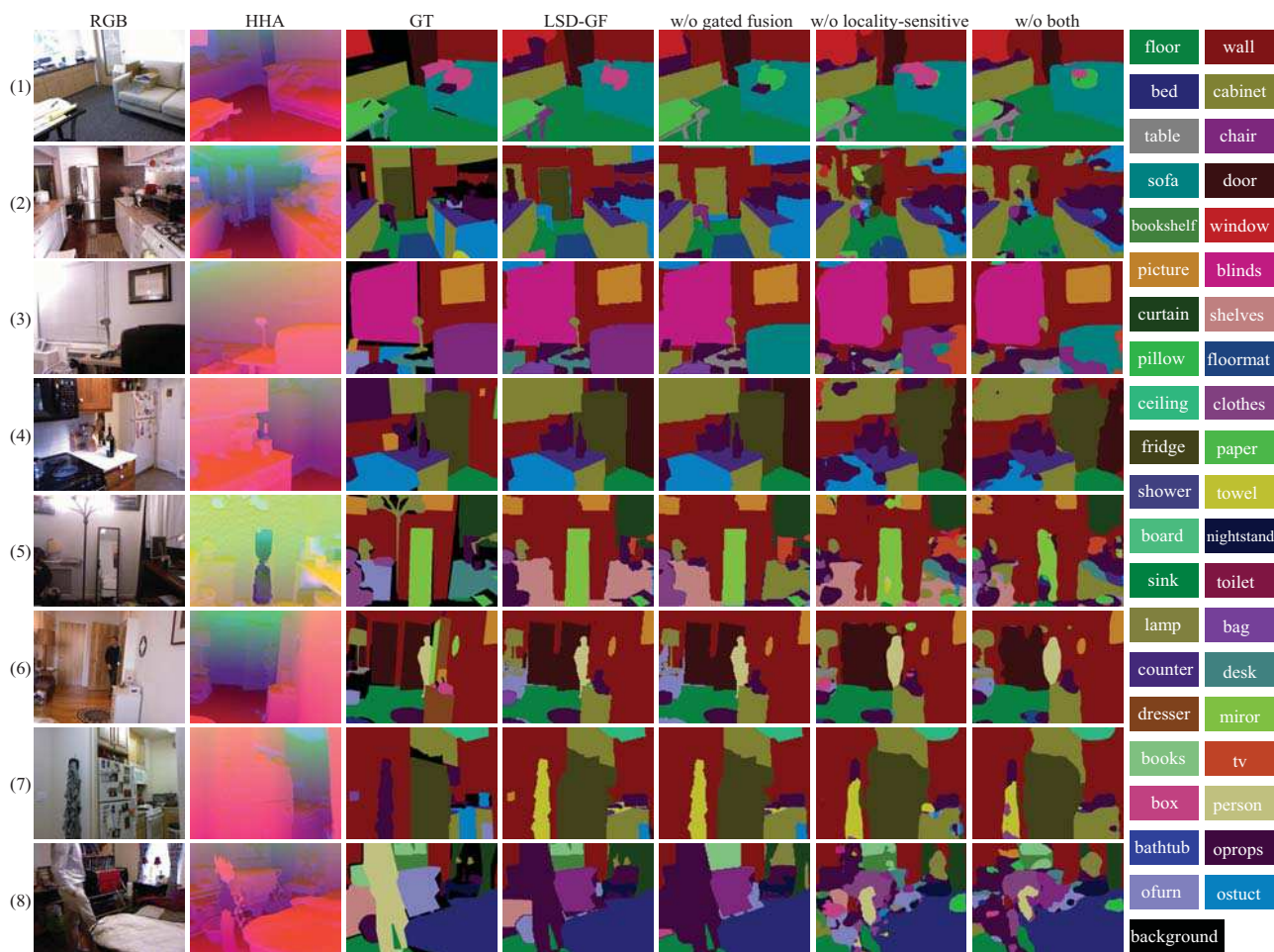
Figure 4. Visual comparison of scene semantic segmentation on the NYU-Depth v2 dataset. For the scene image in each row, we show: (column 1) the RGB image; (column 2) the HHA image; (column 3) the ground truth of semantic segmentation; (column 4) the result of our LSD-GF approach, i.e., l in Table 3; (column 5) the result of LSD-GF whose gated fusion is replaced by sum fusion, i.e., i in Table 3; (column 6) the result of LSD-GF whose locality-sensitive module is removed, i.e., h in Table 3; (column 7) the result of LSD-GF whose locality-sensitive is removed and the gated fusion is replaced by sum fusion, i.e., e in Table 3. See detailed analysis in the text. Best viewed in the magnified color image.
