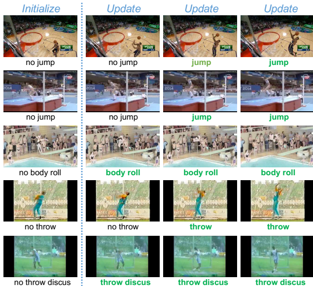
Figure 8. Qualitative results on the MultiTHUMOS validation set. Labels are our model’s predictions for each frame. Our model initializes on the first frame and updates using the next three frames. Our update mechanism correctly recognizes the start of actions after initialization, and even corrects errors from initialization (last).
