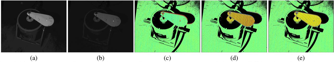
Figure 9. Measurement results of vibrator displacement of vibratory equipment (frequency of vibration : 10 Hz): a) Original image of the object; b) Captured fringe image; c) to e) Phase-shift error images (color bar range from blue (-0.005) to red (0.005) t = 0 msec in c), 30 msec in d), and 60 msec in e))
