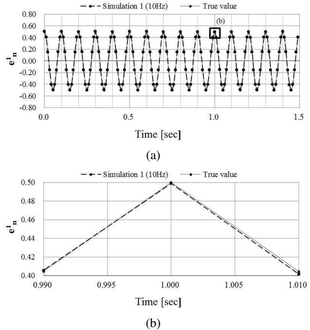
Figure 4. Results of phase-shift error estimation in simulation data (frequency of vibration: 10 Hz): (a) Comparison of estimated phase-shift  $e_1(t)$  and true value and (b) Enlarged view of part of Figure 4 (a).
