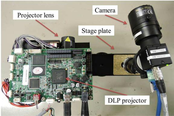
Figure 6. Experiment setup (our systems sensor)
