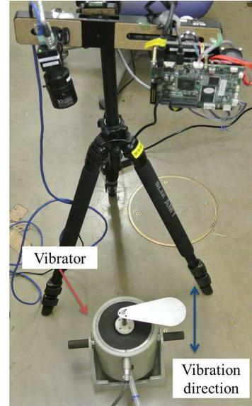
Figure 7. Setup of experiment 1 (vibrator)
