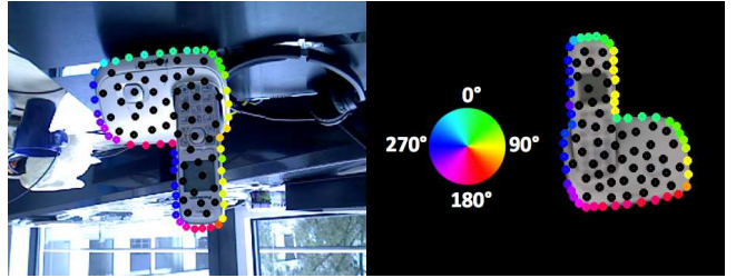
Figure 5. Current tracking and closest pre-rendered viewpoint augmented with contour and interior sampling points. The hue represents the normal orientation for each contour point. Note how we rotate the orientation of each contour point by our approximation of the inplane rotation such that the SDF computation is proper.
