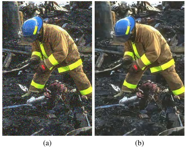
Figure 1. Image denoising with the proposed deep non-local image model. (a) Noisy image corrupted with additive Gaussian noise ( \sigma = 25 ); PSNR = 20.16 dB. (b) Denoised image using the 5-stage feed-forward network described in Sec. 3.3; PSNR = 29.53 dB.
