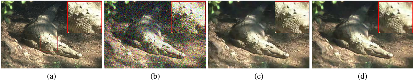
Figure 5. Color image denoising. (a) Original image, (b) Noisy image corrupted with Gaussian noise ( \sigma = 50 ); PSNR = 14.15 dB. (c) Denoised image using \text{CNLNet}_{5 \times 5}^{5 \times 5} ; PSNR = 26.06 dB. (d) Denoised image using CBM3D [7]; PSNR = 25.65 dB.
