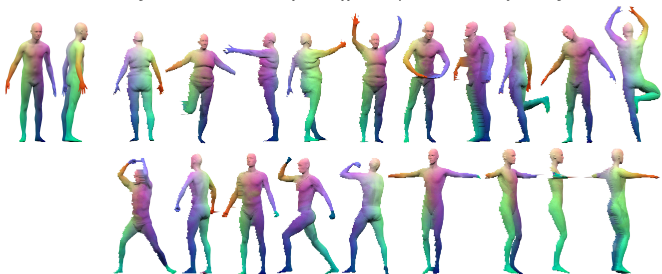
Figure 8. Visualization of correspondence on FAUST range maps as color code (corresponding points are shown in the same color). Full reference shape is shown on the left. Bottom row show examples of additional shapes from SCAPE and TOSCA datasets.
