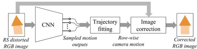
Figure 5. Overview of rolling shutter correction.
