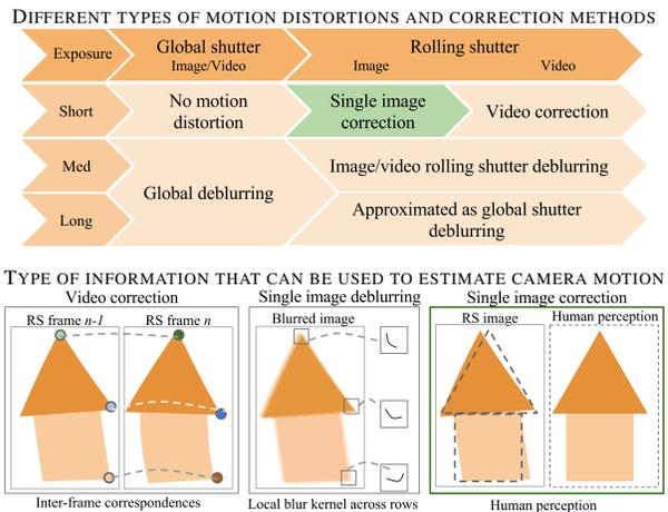
Figure 1. Overview of correction techniques for various image capture and exposure settings.
