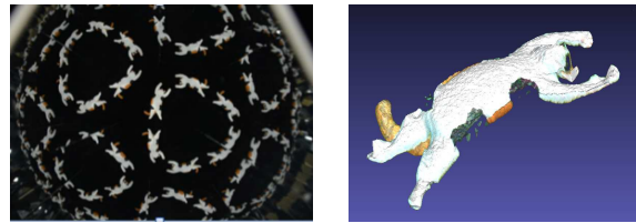
Figure 1: Kaleidoscopic imaging system. Left: kaleidoscopic projection of a 3D cat object. Right: a 3D reconstruction result.
