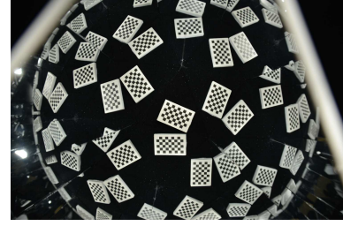
Figure 7: A capture of a chessboard used as the reference object for conventional methods
