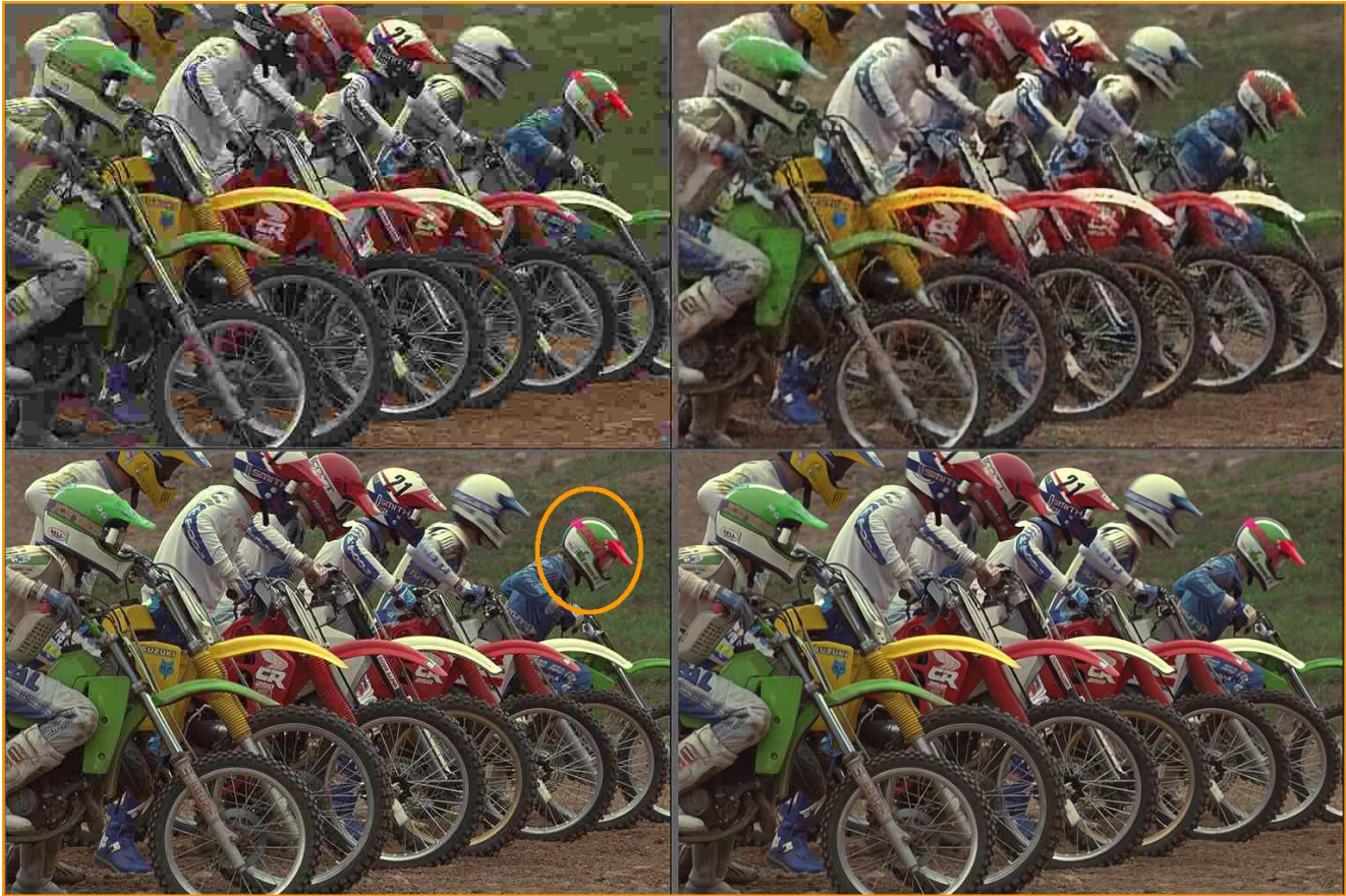
Figure 7. Comparison of compression results on Kodak Image 5. The top row is target at 0.25 bpp, the bottom row at 1.00 bpp. The left column is JPEG 420 and the right column is our Residual GRU (One Shot) method. The bitrates for our method are before entropy coding. In the first row (0.25 bpp) our results are more able to capture color (notice color blocking on JPEG). In the second row (1.00 bpp) our results don't incur the mosquito noise around objects (one example is highlighted with an orange circle). Results at 1 bpp may be difficult to see on printed page. Additional results available in the supplemental materials.
