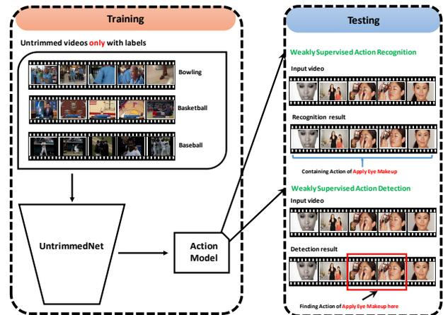
Figure 1. **Weakly supervised action recognition and detection:** during training phase, we simply have untrimmed videos without temporal annotation and we train action models from these untrimmed videos directly; during test phase, the learned action models could be applied to action recognition (WSR) and detection (WSD) in untrimmed videos.
