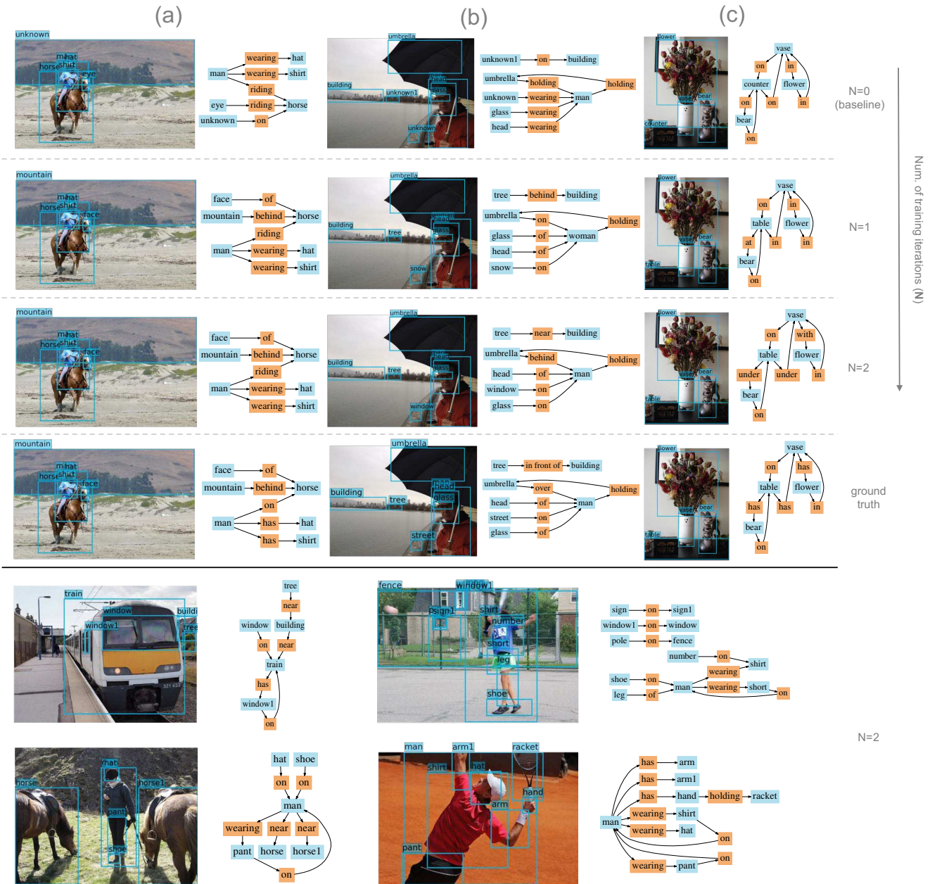
Figure 5. Sample predictions from the baseline model and our final model trained with different numbers of message passing iterations. The models take images and object bounding boxes as input, and produce object class labels (blue boxes) and relationship predicates between each pair of objects (orange boxes). In order to keep the visualization interpretable, we only show the relationship (edge) predictions for the pairs of objects (nodes) that have ground-truth relationship annotations.
