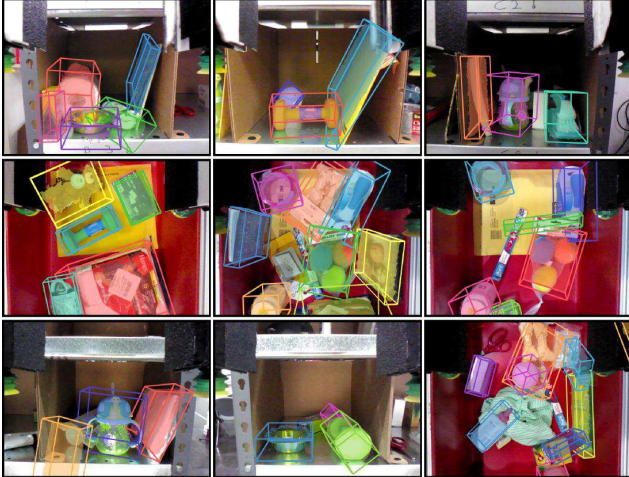
Figure 8. Predicted object poses on the Shelf & Tote Benchmark using 3DMatch + RANSAC. Predicted object poses are shown on the images of the scans with 3D bounding boxes of the transformed object models. 3DMatch + RANSAC works well for many cases; however, it may fail when there is insufficient depth information due to occlusion or clutter (bottom).
