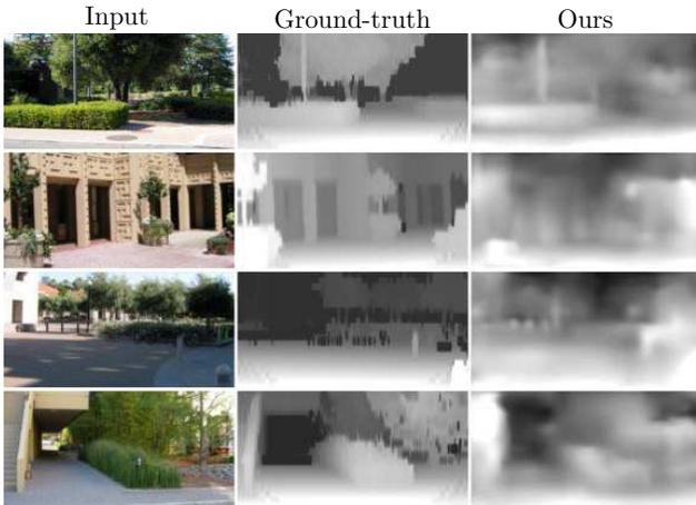
Figure 8. Our sample predictions on the Make3D dataset. Note that our model is trained on KITTI + Cityscapes only, and directly tested on Make3D.
