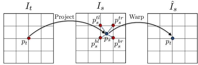
Figure 3. Illustration of the differentiable image warping process. For each point  $p_t$  in the target view, we first project it onto the source view based on the predicted depth and camera pose, and then use bilinear interpolation to obtain the value of the warped image  $\hat{I}_s$  at location  $p_t$ .
