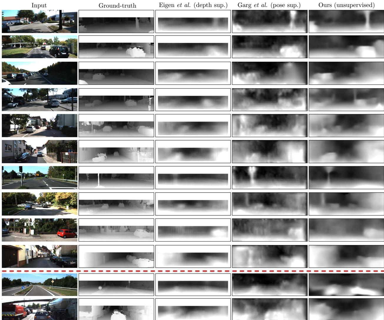
Figure 6. Comparison of single-view depth estimation between Eigen *et al.* [7] (with ground-truth depth supervision), Garg *et al.* [14] (with ground-truth pose supervision), and ours (unsupervised). The ground-truth depth map is interpolated from sparse measurements for visualization purpose. The last two rows show typical failure cases of our model, which sometimes struggles in vast open scenes and objects close to the front of the camera.
