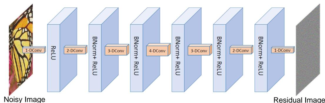
Note that “s-DConv” denotes s-dilated convolution,  $s = 1, 2, 3$  and  $4$ ; “BNorm” represents batch normalization; “ReLU” is the rectified linear units ( $\max(\cdot, 0)$ ).
