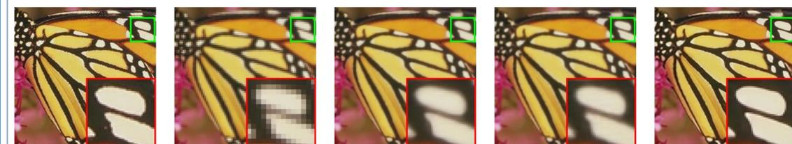
Figure: Single image super-resolution performance comparison for Butterfly image from Set5 (the blur kernel is  $7 \times 7$  Gaussian kernel with standard deviation 1.6, the scale factor is 3). The proposed deep CNN denoiser prior based optimization method can super-resolve LR image by tuning the blur kernel and scale factor without training.
