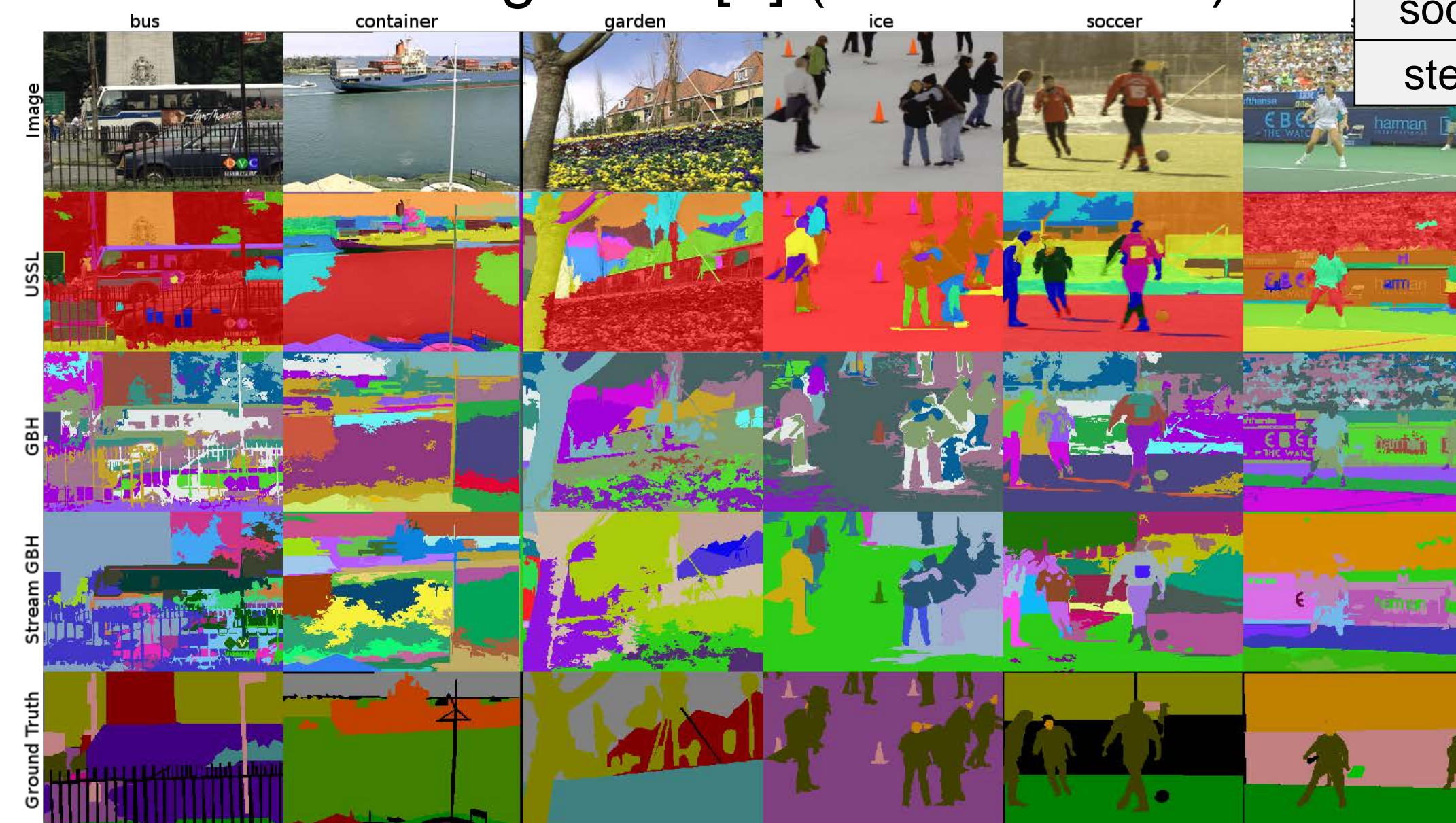
Above: Summary of segmentation output of USSL and the hierarchical graph-based approaches from the level that is most similar to the USSL output. Left: Qualitative comparison of output of each segmentation technique
