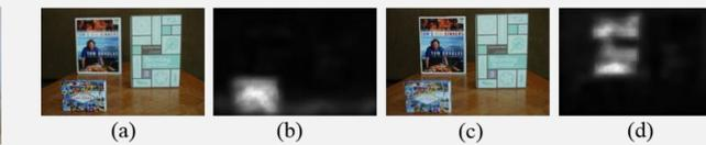
Fig. 5: Application of our method to changing the camera focus and DFF. (a) & (c) are images with different focus areas. (b) & (d) are our estimated maps.
