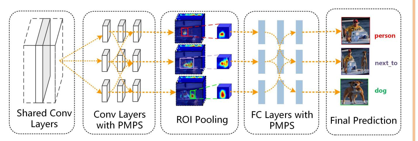
ViP-CNN first generates triplet proposals with RPN and then feeds them into corresponding models. A triplet NMS is proposed to reduce the number of triplets. ROI-pooling is used to generated the features of the fixed size. The three branches are connected at both conv and fc layers using Phrase-guided Message Passing Structure (PMPS). So the three models can make the decision with the sense of the each other. And the final recognition of subject, object and predicate is done simultaneously.
