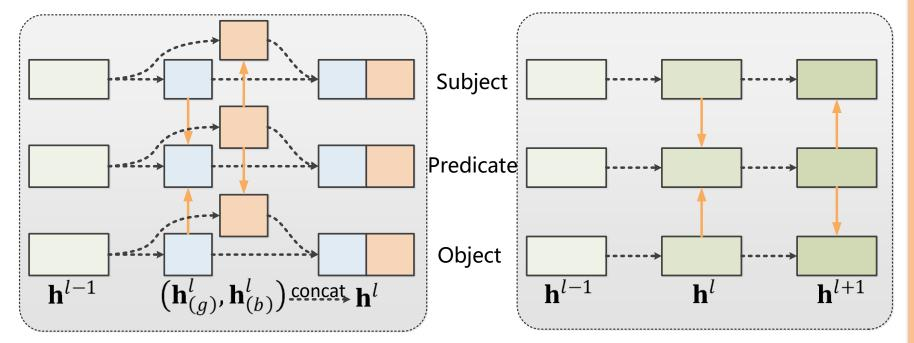
Phrase-guided Message Passing Structure (PMPS) is proposed to employ the complementary effects of simultaneously recognizing the objects and predicates.
