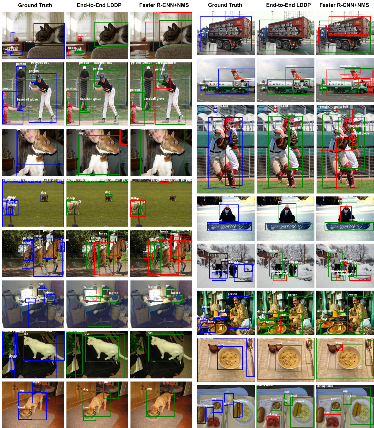
Figure 3: Example images from MS COCO data set illustrating our end-to-end LDDP and Faster R-CNN followed by NMS. A score threshold of 0.6 is used to display images.
