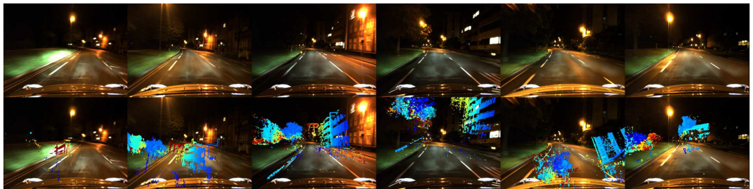
Figure 4. Sample depth maps projected into images during outdoor localisation against a map built at dusk. Key-frame appearance and depth maps are shown at the top, and the results of the NID-SLAM tracking against the key-frame are shown for each of three different conditions (overcast, snow and night), demonstrating robust tracking in the presence of outdoor lighting (overcast to dusk) and weather (snow to spring) changes. Note that NID-SLAM was not capable of localising at night relative to a map built under a different condition.
