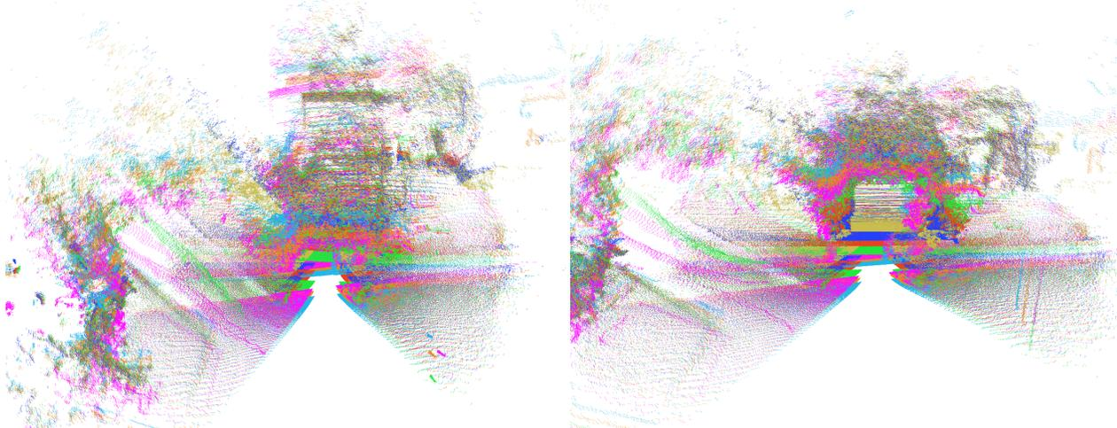
Figure 3: Depiction of the BB-ICP alignment of the first 6 LiDAR scans of the Gazebo Summer dataset [1]. While details of the alignment could be improved, the overall large scale alignment is inferred correctly. Different colors indicate distinct LiDAR scans.
