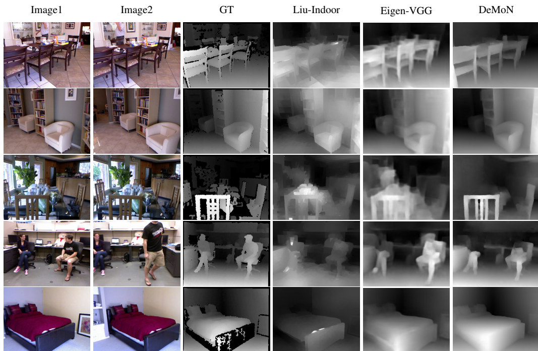
Figure 10. Qualitative depth prediction comparison on NYUv2. The Base-Oracle prediction is not available because there is no motion ground truth. Our method fails to predict the upper bodies of the persons in the fourth example because the persons move between the two frames.
