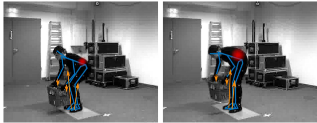
Figure 1. Analysis of lifting motions: Based on 2D motion data we estimate the torque in the lower back for different kinds of lifting motions. In contrast to other approaches we use the laboratory setup only for evaluation. The orange arrows represent modeled outer forces and the red areas the maximum joint torque. Lengths and radii are proportional to the force and torque magnitudes, respectively.
