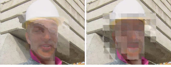
Figure 2: Keeping only the DC of each block of the luminance channel with h = 204 and w = 220 (on the RoI). Blocks size: 4 \times 4 for the right image and 24 \times 24 for the left one.
