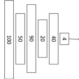
Figure 6: Action recognition component consisting of 6 fully connected layers beginning with a layer of 100 neurons to 50, 90, 20, 40 and ending with a fully connected layer of 4 to perform action recognition.
