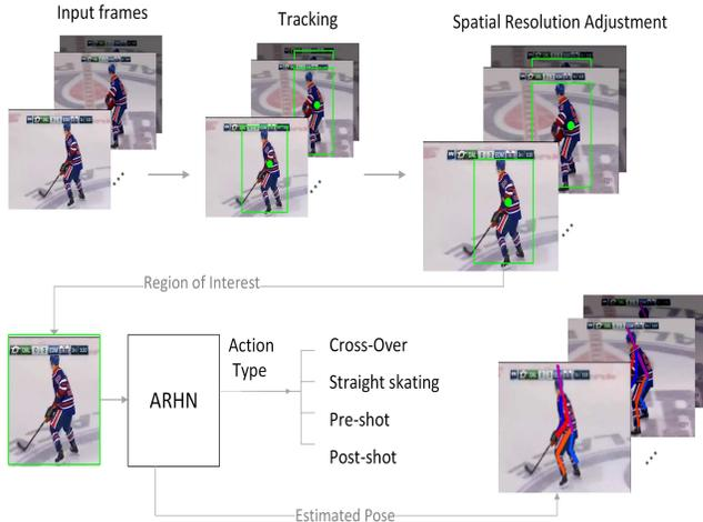
Figure 1: Implemented framework for hockey action recognition through pose estimation for hockey images/video frames. The framework begins by extracting video frames as input, the body-center of the player is determined using tracking means, then the image size is scaled and fed into the network. The network then classifies the action and overlays the estimated pose on the image.
