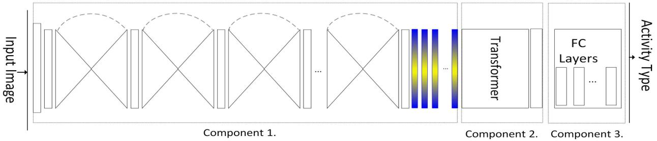
Figure 2: Proposed ARHN for action recognition identifying the three components. Component 1: pose estimation using an hourglass network. Component 2: feature transformation to transform poses into a common frame of reference Component 3: action recognition represented by fully connected layers.
