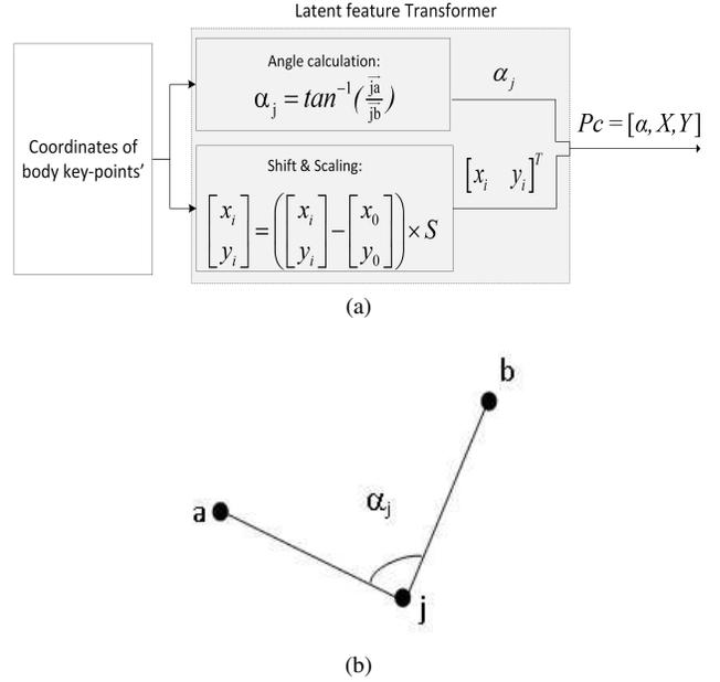
Figure 5: (a) Latent feature transformer, which generates canonical pose vector by shifting and scaling joint coordinates and computing the joint angles. (b) Angle of joint "j" (i.e.,  $\alpha_j$ ) is the smaller angle between vectors ja and jb.
