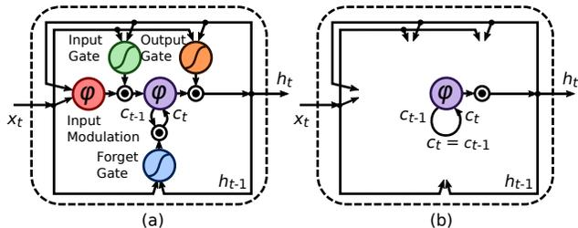
Figure 2. (a) LSTM, (b) LSTM of *Keeping State*
