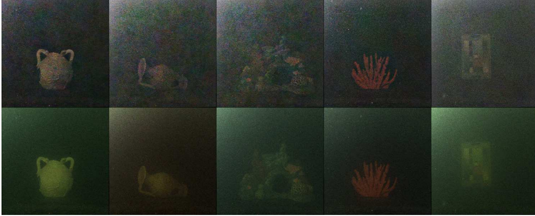
Figure 8. (Top) Intermediate results of our proposed method showing single image dehazing of center sub-aperture image. (Bottom) Comparative results of UDCP, a single image dehazing method based a physical model of image formation underwater.
