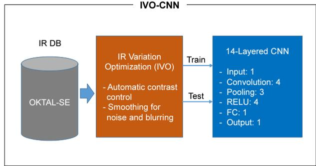
Figure 2. Proposed IR Variation Optimized deep Convolutional Neural Network (IVO-CNN) for automatic ground target recognition with synthetic image generator.
