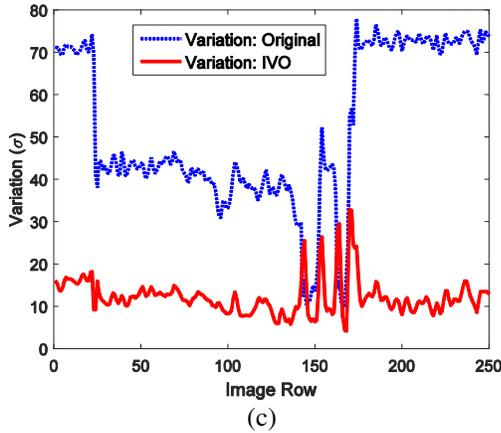
Figure 7. Quantitative analysis of the IR variations for the column sectional data: (a) original IR data, (b) IR data after IVO, (c) comparison of the IR variations in terms of the standard deviation.
