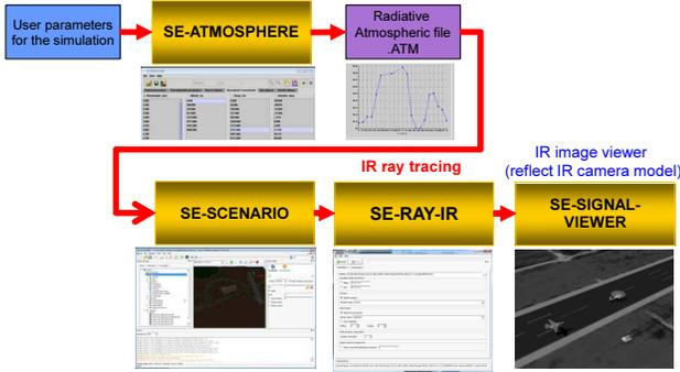
Figure 3. OKTAL-SE-based synthetic IR image generation flow: SE-ATMOSPHERE generates atmospheric data and SE-SCENARIO controls targets and background. SE-RAY-IR synthesize IR images by ray tracing and SE-SIGNAL-VIEWER visualizes the results.
