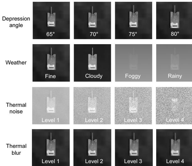
Figure 4. Synthesized IR target examples using the OKTAL-SE for a T72 target by varying the target attributes, imaging geometry, and atmospheric parameters.
