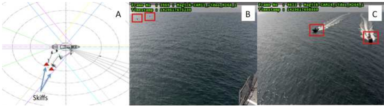
Figure 3. Sc3_Tk1 of the IPATCH-PETS dataset. A) The schematic representation of the scenario indicates two skiffs loitering before speeding up to attack a vessel. B) Two skiffs observed stationary (Loitering) by one of the ship cameras. C) The two skiffs observed speeding up for an attack against the vessel.
