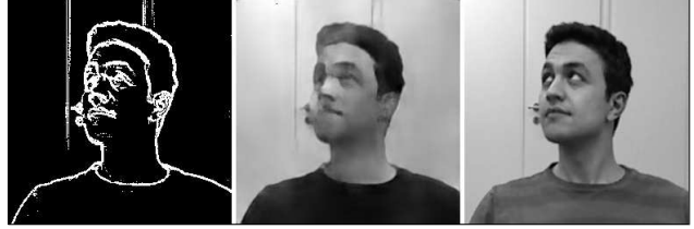
Figure 4: Figure of the intensity reconstruction (middle pane) on the binary data (left pane) simulated from the BIWI dataset [5]. The ground truth is on the right.
