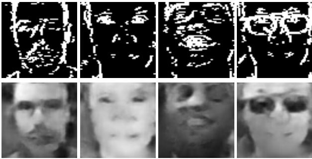
Figure 8: Intensity reconstruction result inferred by the network described in Section 3.2 and trained on the WIDER simulated data. The top row shows 64x64 face crops captured with the prototype camera, the bottom the corresponding reconstructed images. While the quality is not quite on par with the intensity reconstructions, it has to be noted that the resolution of the crops in Figure 5, is 96x96, i.e. 1.5x larger.
