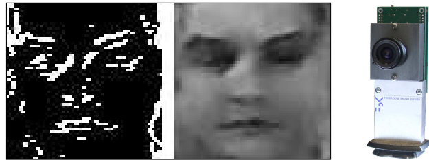
Figure 1: Figure showing a captured binary spatial gradient video (left), our intensity reconstruction (middle), and the prototype camera we used for the capture.
