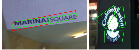
Figure 7. Failure cases of our method. The boxes in green are ground truth. The red boxes are our predictions.
