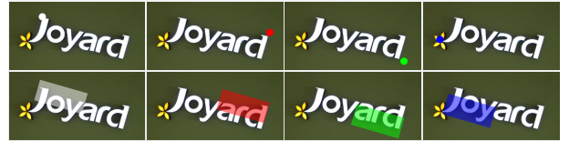
Figure 1. The images in top row and bottom row are the predicted corner points and position-sensitive maps in top-left, top-right, bottom-right, bottom-left order, respectively.
