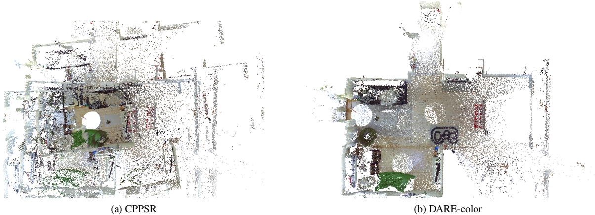
Figure 5. Joint registration of the four point sets in the VPS indoor dataset. (a) CPPSR [6] only aligns the high density regions and neglects sparsely sampled 3D-structure. (b) Corresponding registration using our density adaptive model incorporating color information.
