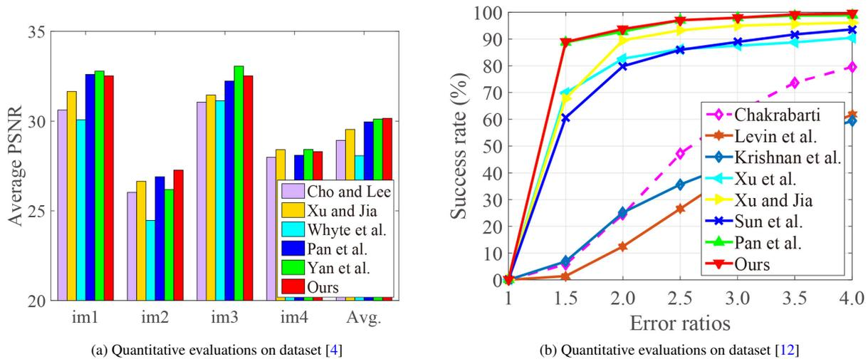
Figure 5. Quantitative evaluations on the benchmark datasets [4, 12]. The dataset by Köhler et al. [4] contains 48 blurred images, including 4 clear images and 12 challenging blur kernels. Our method generates results having the highest average PSNR among other state-of-the-art methods. The dataset by Sun et al. [12] contains 640 blurred images including 80 clear images and 8 blur kernels from [6]. Our method performs favorably against state-of-the-art methods.
