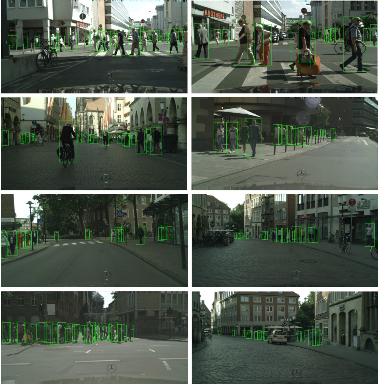
Figure 2. More examples on CityPersons dataset. Green bounding boxes are predicted pedestrians whose score ( [0, 1.0] ) is greater than 0.8.
