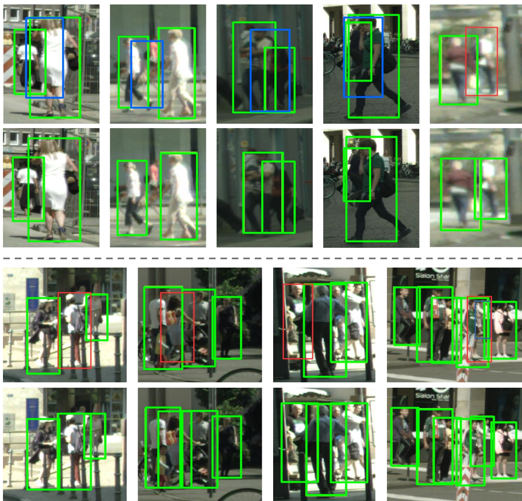
Figure 1. Comparison of baseline and RepLoss. The blue bounding boxes represent false positives, and the red ones represent the missed detections. On two sides of the grey dashed line, samples on the first row of each side are predictions of our baseline, while samples on the second row of each side are the predictions after adding the RepLoss.
