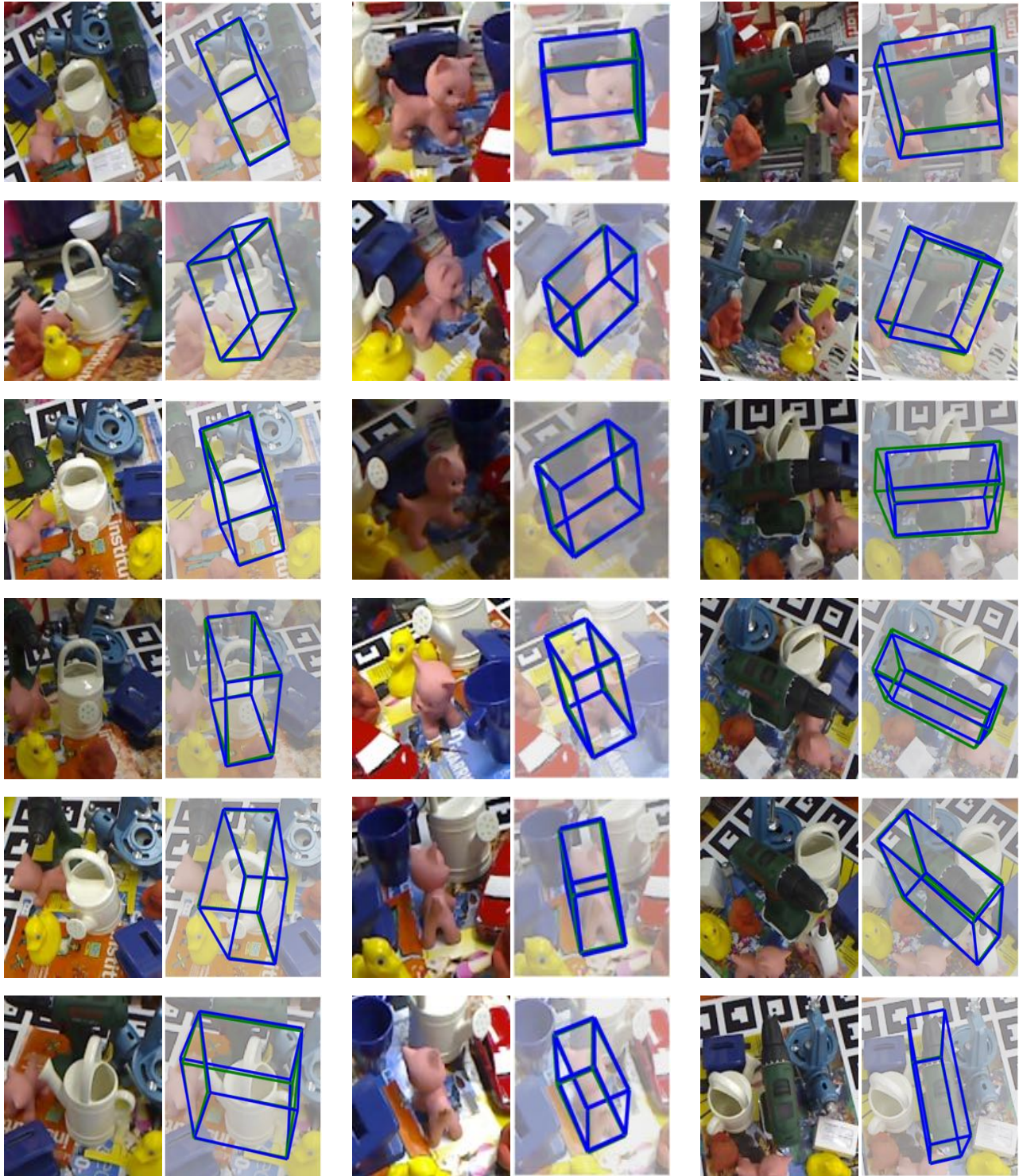
Figure 7. Example results on the LINEMOD dataset: (left) CAN, (middle) CAT, (right) DRILLER. The projected 3D bounding boxes are rendered over the image and they have been cropped and resized for ease of visualization. The blue cuboid is rendered using our pose estimate whereas the green cuboid is rendered using the ground truth object pose. Note that the input image dimension is 640 \times 480 pixels and the objects are often quite small. Noticeable scene clutter and occlusion makes these examples challenging.
