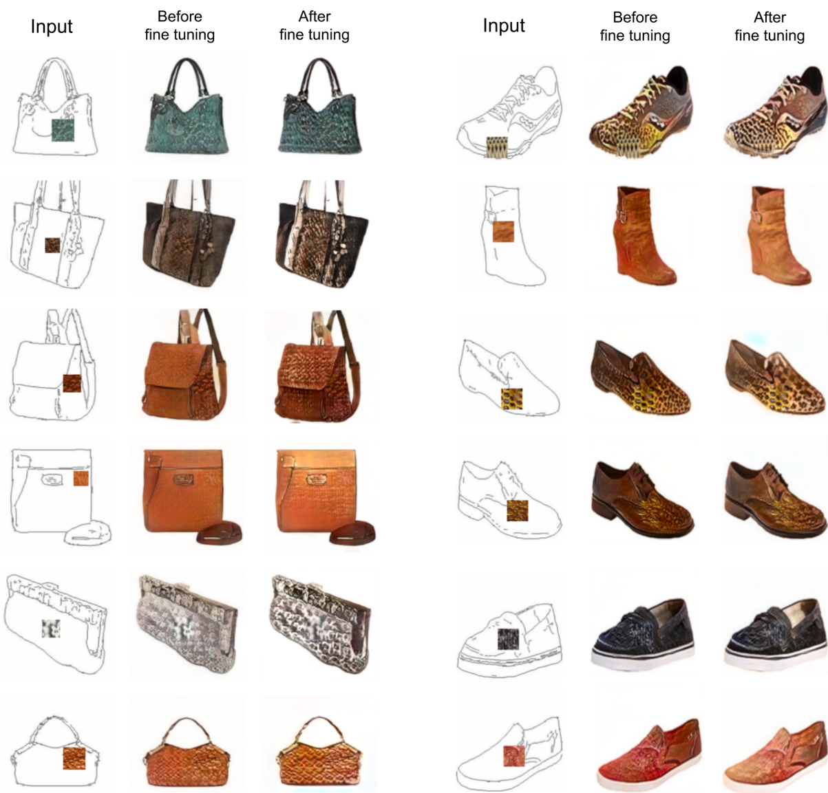
Figure 4: Comparison of results before and after fine-tuning on an external texture database. The base model is trained on handbag and shoe sketches with ground truth images. The fine-tuned model with local texture loss improves texture propagation on difficult texture with high contrast and strong regularity, e.g. striped, dotted, checkerboard patterns, which are rarely seen in the ground-truth.
