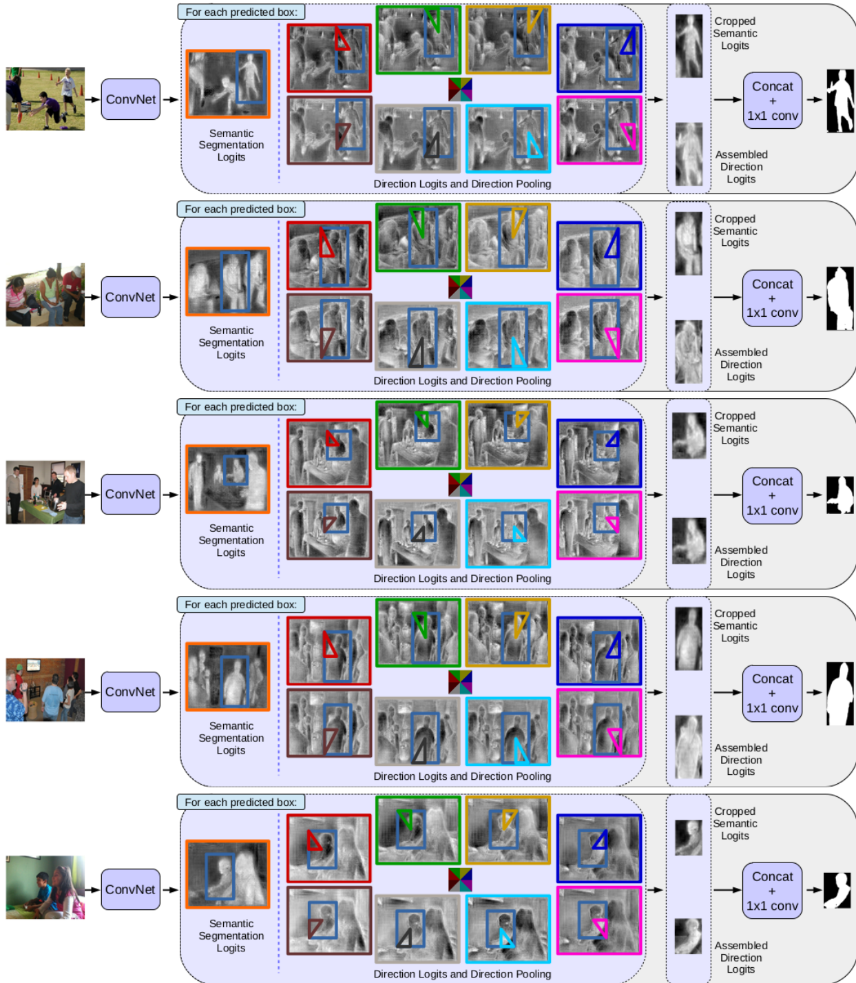
Figure 1. Semantic segmentation logits and direction prediction logits are used to perform foreground/background segmentation within each predicted box. In particular, segmentation logits are able to distinguish instances of different semantic classes ( e.g. , person and background), while direction logits (directions are color-coded) further separate instances of the same semantic class ( e.g. , two persons in the predicted box). In assembling operation, regional logits (the color triangular regions) are copied from each direction channel.
