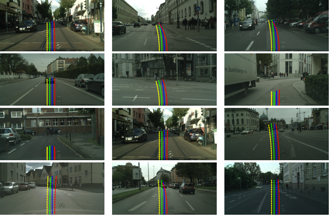
Figure 2: Odometry prediction: We show predicted odometry for 15 time-steps as points (bottom to top) over-layed on the last visual observation. The distance and angle between subsequent points is the predicted (proportional) speed and steering angle. Color codes: Blue : Ground-truth, Red : Kalman Filter, Yellow : Our LSTM without visual input, Green : Our LSTM with visual input.
