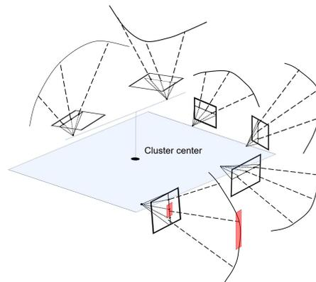
Figure 1: Due to radial distortion, rows of rolling shutter images correspond to rays which span a curve in space. Rolling shutter further provides a dense sampling of the scene in time. This combination of high frequency and curved sampling of the scene provides us more information than traditional pinhole cameras. The highlighted region reflects per-row image region corresponding to the curve.
