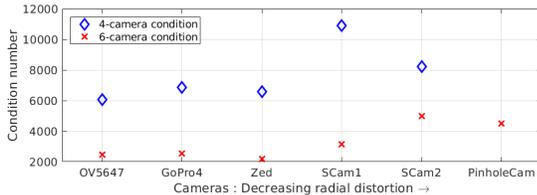
Figure 3: With higher radial distortion, the system stability increases (smaller condition number). Additional views increase stability (4- vs. 6-cameras). The plot shows the worst-case condition number (PinholeCam 4-camera result too large to show).
