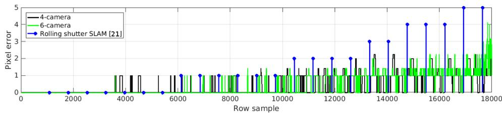
Figure 7: Render pixel estimates: Our 4-camera configuration (black) has higher error than our 6-camera configuration (green). Blue dots show the rendering error obtained by the method of Kim *et al.* [21], which maintains a pose estimate per keyframe, rather than per row.
