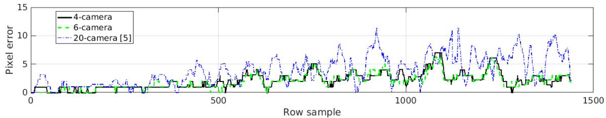
Figure 4: For the same camera motion, our tracking incurs far smaller rendering pixel errors using only 4 cameras as opposed to the 20-camera system of [5] for synthetic data.
