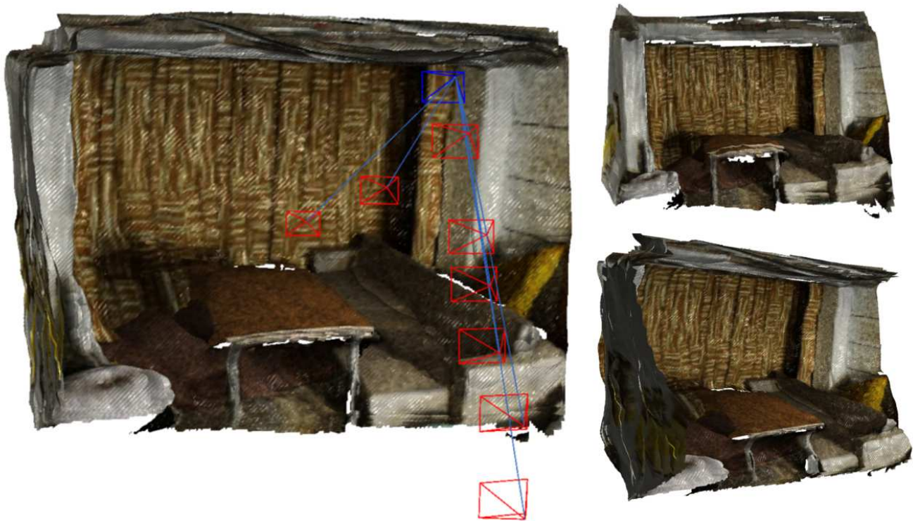
Figure 9. Monocular 3D reconstruction using 9 keyframes. During optimisation a selected master keyframe is paired with the other frames. The depth images of all frames are used for the 3D rendering. The employed geometric error term ensures the consistency between the depth of the different views.
