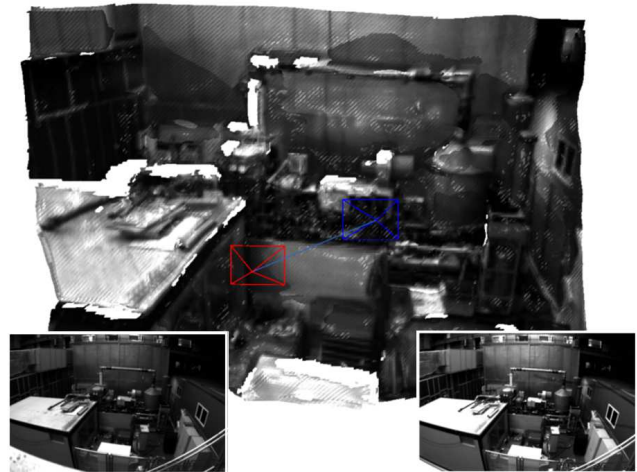
Figure 1. Two view reconstruction on selected frames from the EuRoC dataset. The proposed compact representation of 3D geometry enables joint optimisation of the scene structure and relative camera motion without explicit priors and in near real-time performance.
