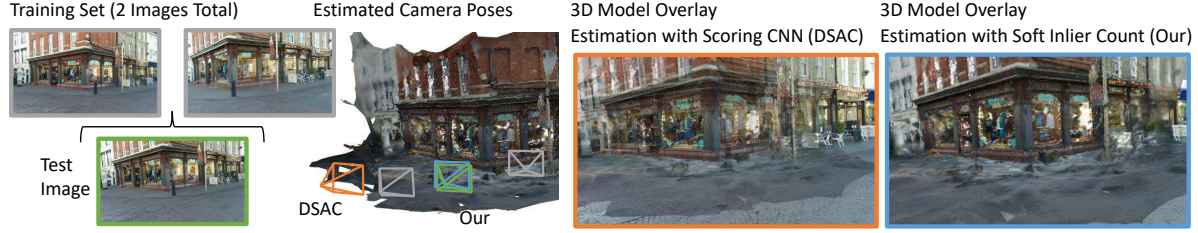
Figure 3. Generalization Capabilities. We train two CNNs for scene coordinate regression and pose hypothesis scoring following DSAC [2] but using only two training images (gray). The system cannot generalize to an unseen test image (green), and produces an estimate far off (orange, 3.7m and 12.6° pose error). Exchanging the scoring CNN for a soft inlier count (see Sec. 2.3), we obtain an accurate estimate (blue, 0.1m and 0.3° pose error). Note that, apart from the scoring function, we fix all components of the test run, including pose hypotheses sampling. This experiment illustrates that scene coordinate regression generalizes well, while score regression does not.
