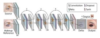
Figure 5: Generator Architecture. For generator G, we use DRN [25] with 3 dilated residual blocks to retain small spatial information (such as eye makeup). d indicates the dilation factor. We use two degridding layers (a 2-dilated  $3 \times 3$  convolution and a  $3 \times 3$  convolution) at the end of the network to avoid grid artifacts. The architecture of F is similar. The only difference is that it takes one image as input and therefore does not need concatenation.
