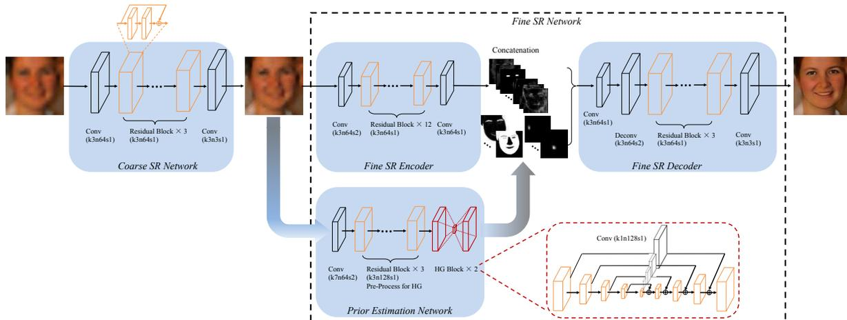
Figure 2: Network structure of the proposed FSRNet. ‘Conv’ indicates a convolutional layer with “pre-activation” structure [11]. ‘k3n64s1’ indicates the kernel size to be  $3 \times 3$ , the feature map number to be 64 and the stride to be 1.
