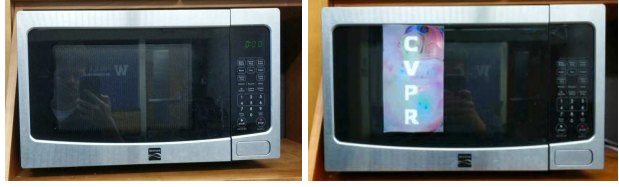
Figure 3: Physical adversarial example against the Inception-v3 classifier. The left shows the original cropped image identified as microwave (85.2%) while the right shows the cropped physical adversarial example identified as phone (77.8%).
