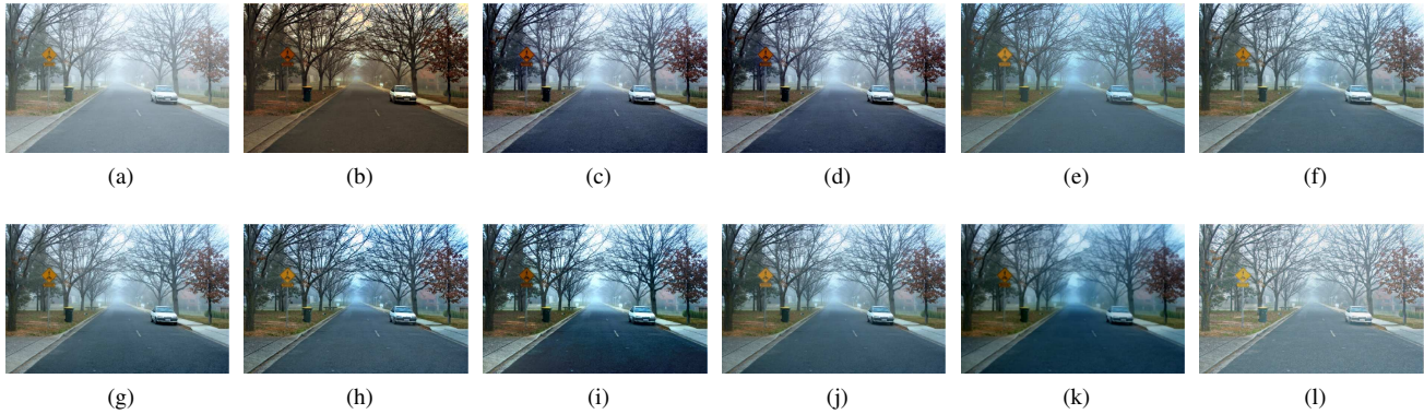
Figure 5. Results of Dehazing by means of Retinex on inverted intensities (marked with asterisk and boldface) as compared to several popular Image Dehazing techniques. (a) Original (b) MSR* [18] (c) RSR* [36] (d) LRSR* [1] (e) HF* (f) WVRI* [12] (g) DCP [17] (h) BCCR[32] (i) DEFADE [7] (j) CAP[52] (k) RAS[6] (l) FVR[46].
