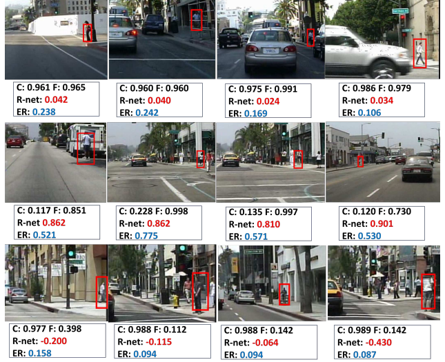
Figure 5: Qualitative comparison of R-net and ER on the Caltech Pedestrians test set. The first row of numbers indicate probability of the red box being a pedestrian. C denotes coarse detection and F indicates fine detection. Red font denotes the accuracy gain of R-net and blue font is for ER. Positive and negative values are normalized to [0, 1] and [-1, 0] . Compared to ER, R-net gives lower positive scores (row #1)/ negative scores (row #3) for regions that coarse detections are good enough/ better than fine detections and it produces higher scores for regions (row #2) where fine detections are much better than coarse ones.
