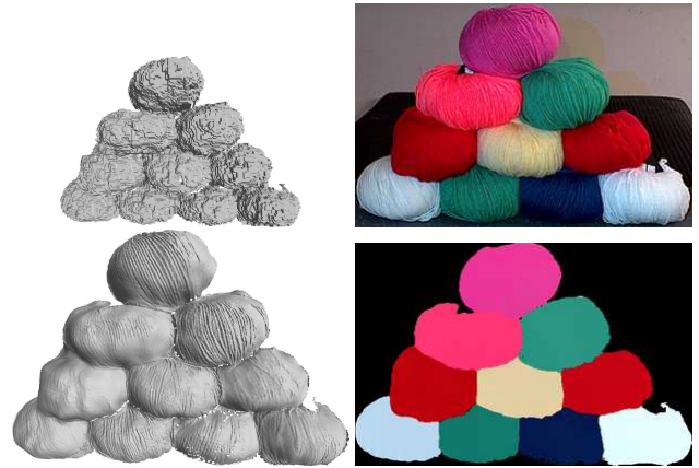
Figure 10: Super-resolution of “wool balls”. Minimal surface drives super-resolution when color gets saturated.
