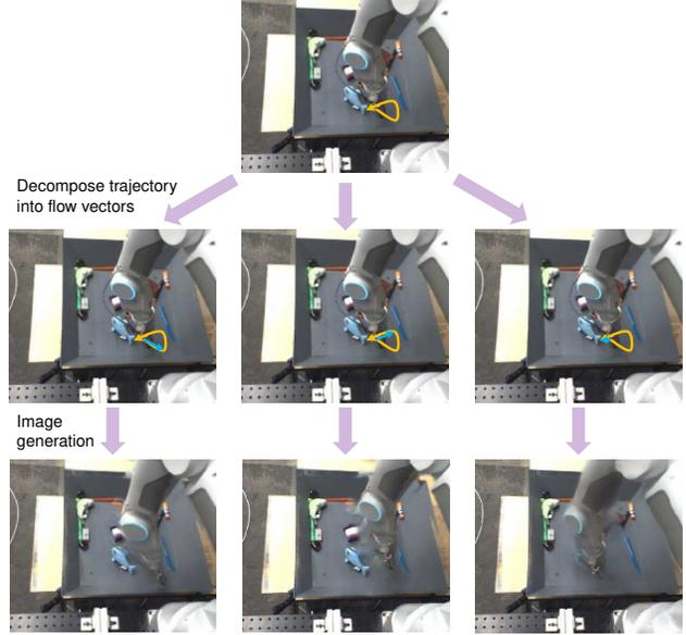
Figure 3. **Generating videos with the image generation model.** Given an input image and a set of trajectories (we only show a single yellow one here for simplicity), we move the end points of the flow vectors (blue vectors) along each trajectory. We then use our image generation model to produce a sequence of frames from the same input image and different flow vectors.
