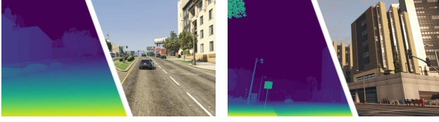
Figure 4. Samples from the proposed MVS-SYNTH dataset, which provides photorealistic images with ground truth disparities even for the sky, reflective surfaces, and thin structures.
