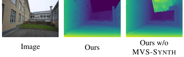
Figure 10. Comparisons between networks trained with and without the MVS-SYNTH dataset. Without MVS-SYNTH dataset, the network has difficulty in handling regions such as the sky because real-world datasets do not cover these regions.
