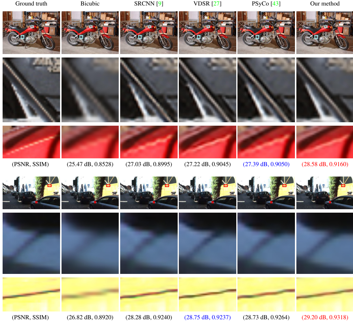
Figure 9: Results of super-resolution with the \times 2 magnification factor. PSNR and SSIM values are shown under each result. The red color indicates the highest PSNR and SSIM values, and the blue color represents the second highest values.
