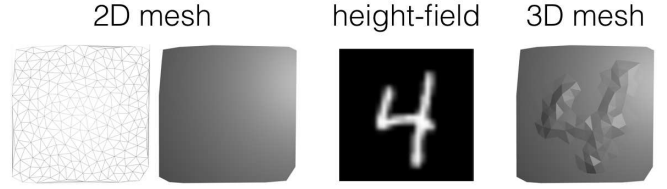
Figure 1. Height-Field Representation of surfaces. A 3D mesh \mathcal{M} \subset \mathbb{R}^3 (right) is expressed in terms of a “sampling” 2D irregular mesh \tilde{\mathcal{M}} \subset \mathbb{R}^2 (left) and a depth scalar field f : \tilde{\mathcal{M}} \rightarrow \mathbb{R} over \tilde{\mathcal{M}} (center).
